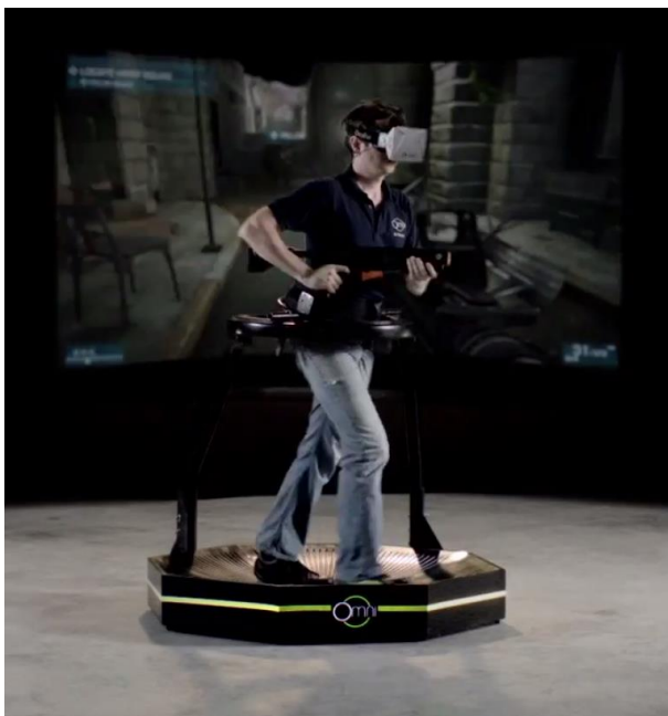
Figure 10 (left) Virtuix Omni treadmill and harness for virtual reality
