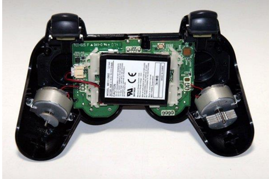
Figure 4 Sony's DualShock 3 controller with two haptic feedback motors in the hand grips exposed
